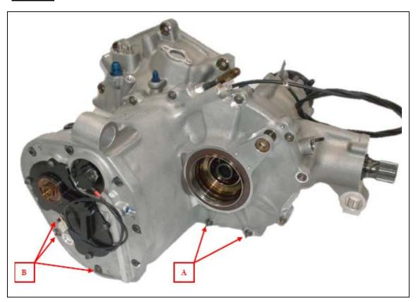
A / B = FIA sealing tag + 2 aluminium seals C= 2 aluminium seals
