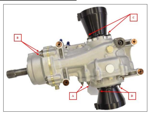
A / B = FIA sealing tag + 2 aluminium seals C / D / E = 2 aluminium seals
