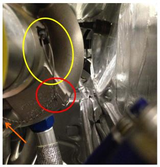
4-make a loop to take the screw on the dashboard side (in yellow on the photo).
