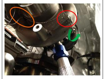
3-drill the compressor housing with the about 2,5 mm-size drill bit as shown on the photo (in red), and then wrap the wire and pass it through.
